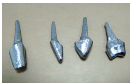
Figure 5. Stump pin inserts moulded from cobalt-chromium alloy Slika 5. Voštani model kočica izliven od legure kobalt-hrom
